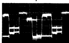
8. TP 17 (IC601 PIN 24) (E-PCB) 4.0V, 10 \mu s / Div
