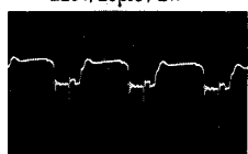
16. Q501 Base (E-PCB) Horizontal Out 10V, 20 \mu s / Div
