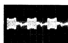
5. IC601 Pin 38 (E-PCB) R - Y In 180mV, 20 \mu s / Div
